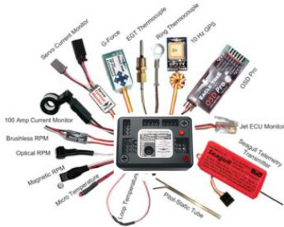
Fig. 12 Flight Data Recorder system
